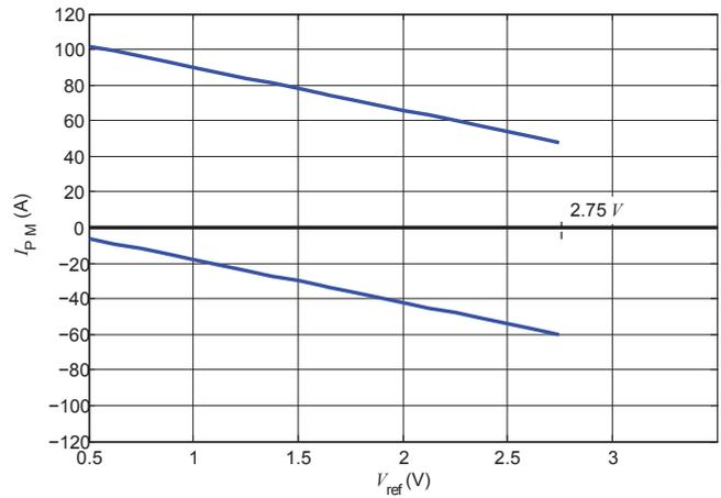
Figure 31: Measuring range versus external  $V_{ref}$  LPSR 15 A
