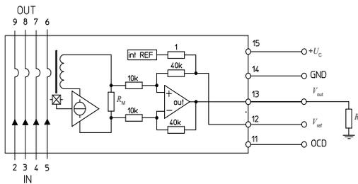
Figure 27: Test connection
