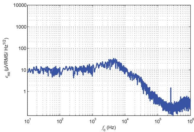
Figure 4: Output noise voltage spectral density
