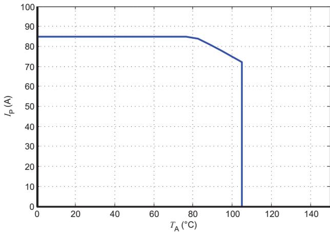
Figure 23:  $I_p$  vs  $T_A$  for LPSR 25-NP
