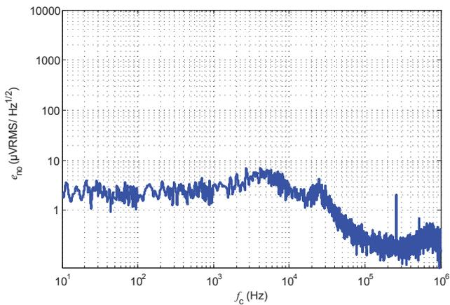
Figure 14: Output noise voltage spectral density
