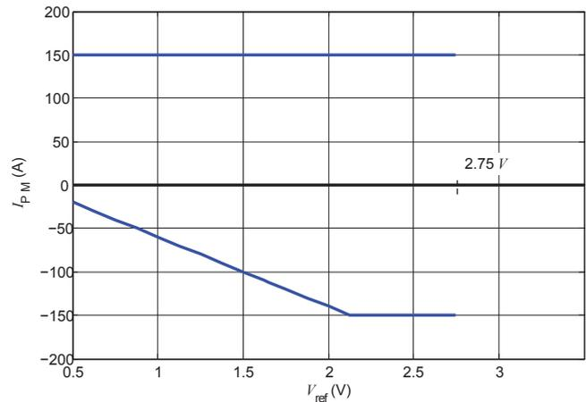
Figure 33: Measuring range versus external  $V_{ref}$  LPSR 50 A
