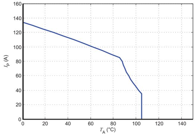
Figure 24:  $I_p$  vs  $T_A$  for LPSR 50-NP
