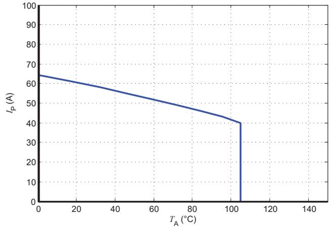
Figure 22:  $I_p$  vs  $T_A$  for LPSR 15-NP
