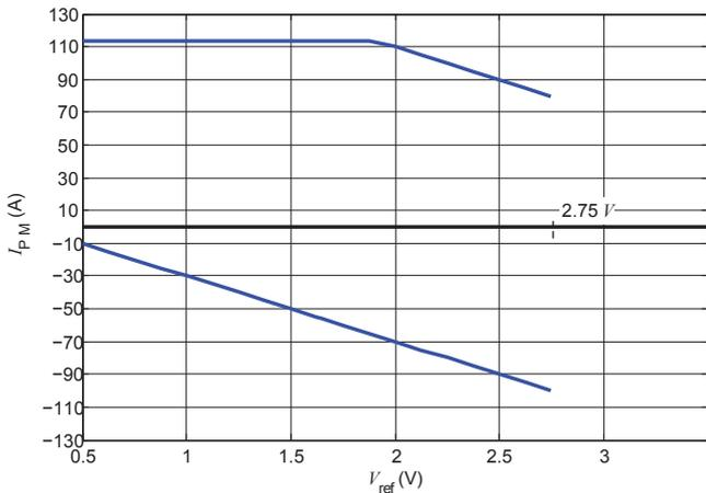
Figure 32: Measuring range versus external  $V_{ref}$  LPSR 25 A
