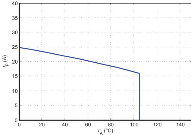
Figure 21:  $I_p$  vs  $T_A$  for LPSR 6-NP
