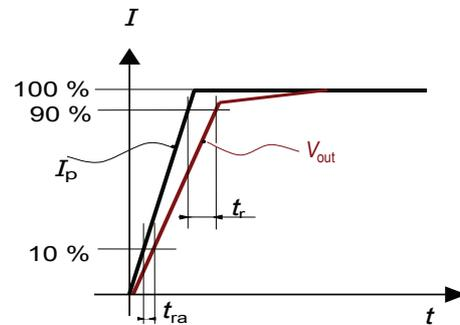
Figure 28: Response time  $t_r$  and reaction time  $t_{ra}$
