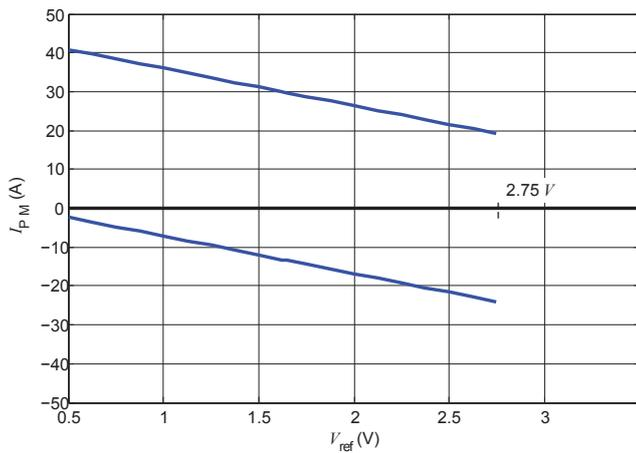
Figure 30: Measuring range versus external  $V_{ref}$  LPSR 6 A
